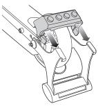
**2** Place a new cartridge in back of the bracket making sure to align the slots on the cartridge with the two legs of the bracket. Slide cartridge forward until you hear a click and the thumb tabs are locked in place.
