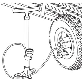
**1** Using a bicycle style tire pump equipped for a Schrader-type valve, inflate the tires to the PSI indicated on the sidewall of the tires.
