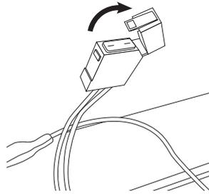
**2** Open fuse box located on the battery.
