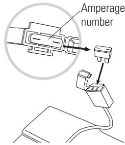
**3** Remove fuse and replace with a new one of equal amperage.
