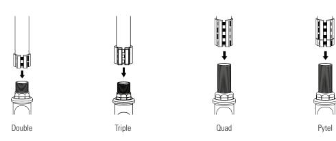
**1** Loosen the collar clamp and slide it upward, Insert T-bar into the fork until it bottoms out on the headset locknut. **Note:** if necessary, carefully twist the T-bar clock-wise while pushing downward until T-bar bottoms out on the headset locknut.
