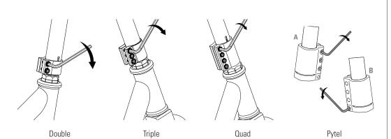
**2** With the front wheel pointed straight ahead, the handlebars square to the front wheel and the Razor logo facing the front (see page 5), tighten the clamp as shown. Alternately tighten each bolt until the clamp is tightened securely.
