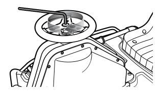
2 Using a 6 mm Allen wrench, tighten the steering bolt to secure the steering wheel in place.
